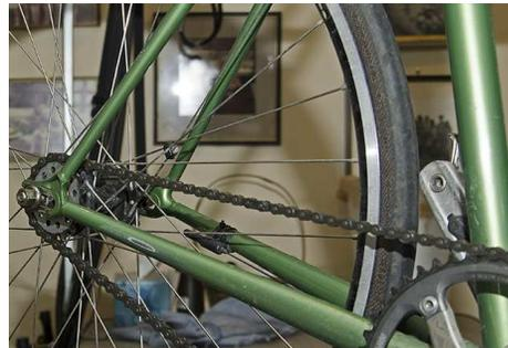
*Fixed-gear Drivetrain and Horizontal Dropout*
